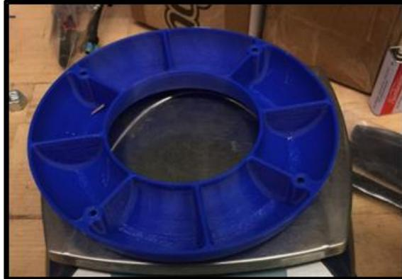
**Figure 2: Vehicle Ballast Ring**
