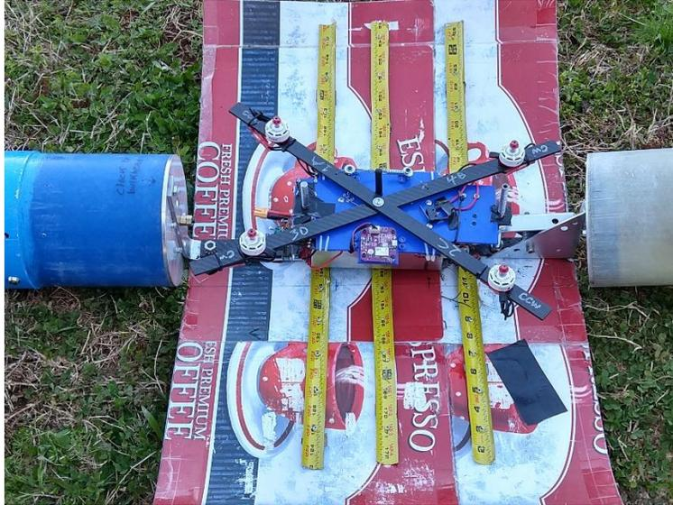
**Figure 5: Deployed Payload After Black Powder Test**
