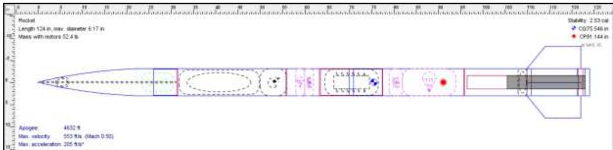
**Figure 2: OpenRocket Model of *ShredIt 40,00***
