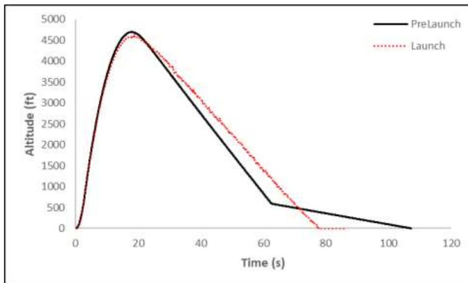
**Figure 3: Pre-Launch Simulation and Actual Launch Data**
