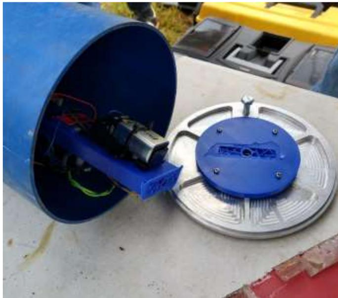
**Figure 6: Nose cone avionics mount post-landing**
