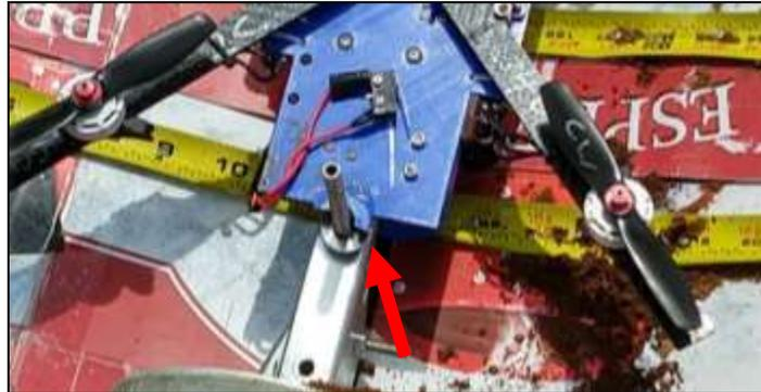
**Figure 7: Damage to UAV Aft Retention Ring**
